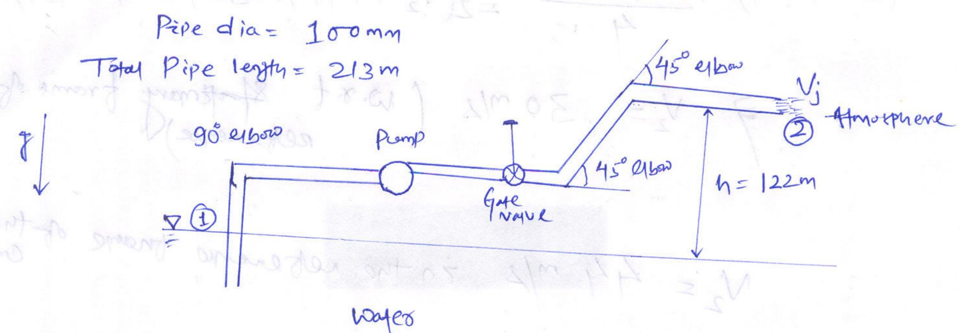
Minor Loss: ① Entrance ② 90° 21600-1 ③ Gate Valve ④ 45° 2160-2 Applying Snergy D-yangle between ① and ②  $\frac{P_1}{g} + q \frac{V_1^2}{2} + g \mathcal{R}_1) - \left(\frac{p_2}{g} + q_2 \frac{V_2}{2} + g \mathcal{R}_2\right) \\
